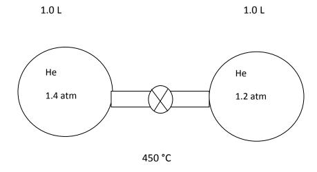
What is the final pressure in the above apparatus if the valve connecting the two bulbs opens (assume negligible volume of the valve) allowing both bulbs filled with He to mix. Assume ideal gas behavior and constant temperature.
